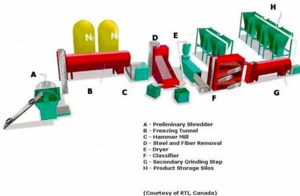
FIGURE 7 Example of a cryogenic [scrap tire] recycling system
